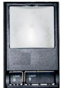
Figure 1 (Sample Garage Door Opener Controller)
